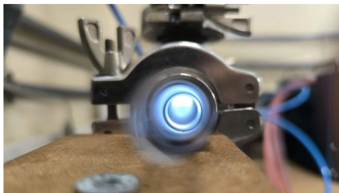
Figure 1 - Microwave discharge ignited at approximately 5 mbar, simulating the atmospheric pressure of Mars.
